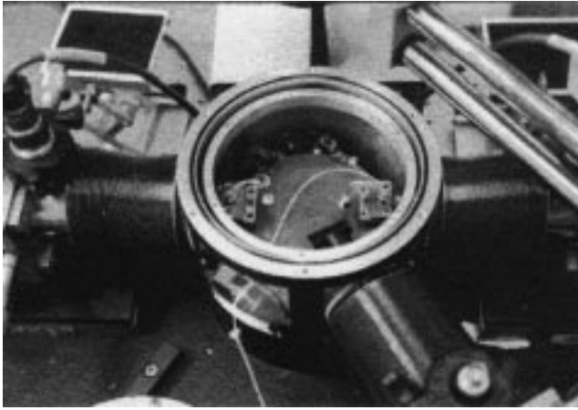
Fig. 1. Photograph of the cryogenic microwave probe station.
